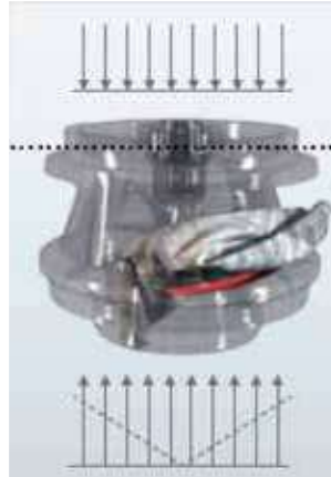
Figure 11: Force distribution when debris enters the pump
