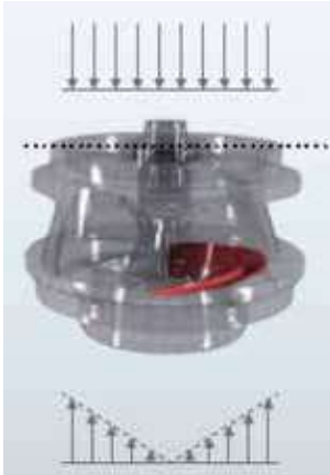
Figure 10: Force distribution during normal operation
